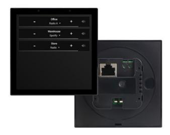
ACW-05 is a networked wall plate controller for the APEX installation amplifiers. A simple 4" touchscreen interface provides non-technical operators with level metering and control over source selection, volume, and mutes for one or more audio zones.
