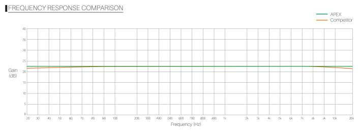
In the comparison frequency response, we can see that both responses are nearly flat apart from a slight roll-off at the high and low extremes. This is more than sufficient flat to power a speaker with an intended response from 60Hz-16K. The Apex GlidePath architecture has a -3dB point of 2Hz, the competitor has a -3dB point of 15Hz.
