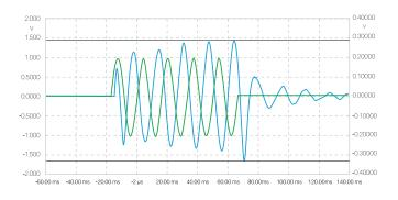
Competitor module driven with a 50Hz 5 cycles burst. This module has a peak cone excursion off +287mV and-328mV. The trail output after the signal stops has a peak output of 100mV
