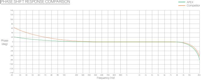
From the phase response curves we see more phase shift with the competitor (red line) due to the DC coupling within the amplifier system.
