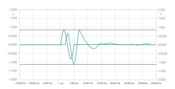
Green line: competitor 200hz 1 cycle. Blue line: actual cone excursion. At the first part of the sine, the cone goes up to 0,64V and drops down to -1,13V in the second part and goes up again to 0,82V as the signal stops.
