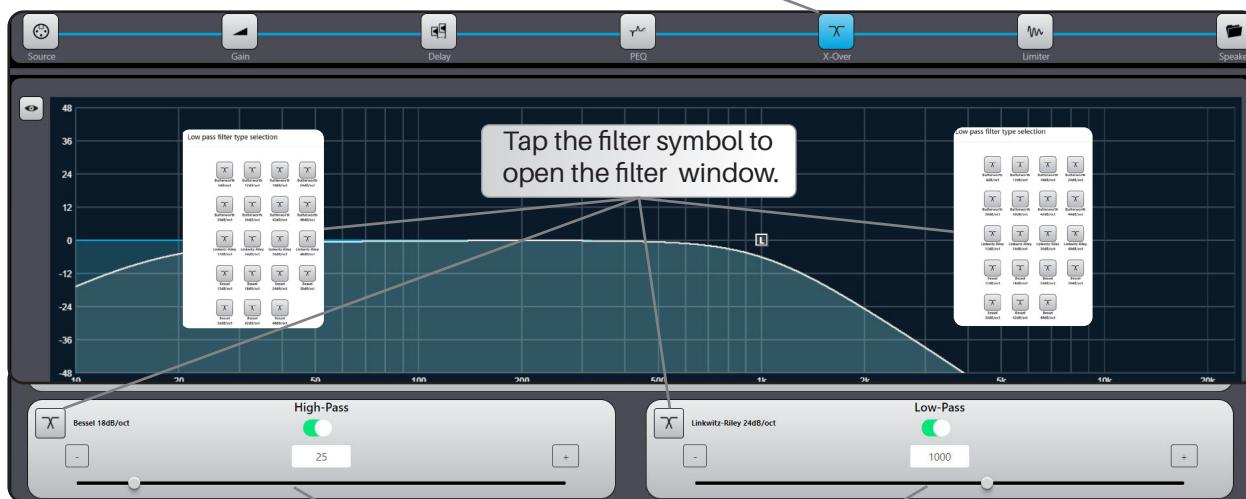
Adjusting the Filter parameters can be done in multiple ways: use the sliders and tap the +/- buttons for fine adjustments or use the on screen drag function with mouse, pen or finger gestures.
