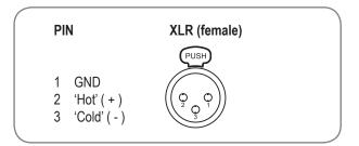
② Output 1 L & R. Outputs are on 3-pin male XLRs, with separate connectors for left and right channels. The outputs are electronically balanced. The pinout is as shown below:
