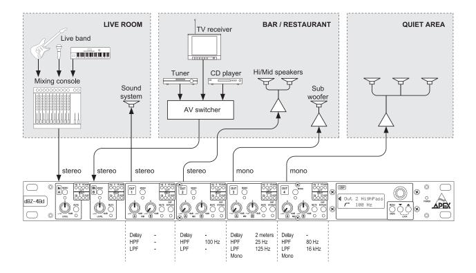
This application uses the dBZ-48d as a 3-way zoner, with two outputs being used to derive LF and HF feeds for a two-way speaker system in one area. The set-up would be suitable for a small venue which features live music in a main area, while a CD player, music server, TV sound or similar is made available at different levels in other rooms.
