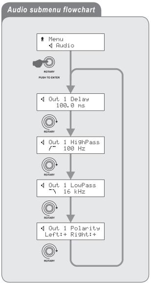
Once the first submenu item is displayed, the rotary encoder can be used to step through the others; to select an item, press **Enter** while it is displayed.
