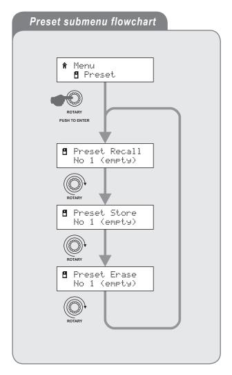
Once the first submenu item is displayed, the rotary encoder can be used to step through the others; to select an item, press Enter while it is displayed.
