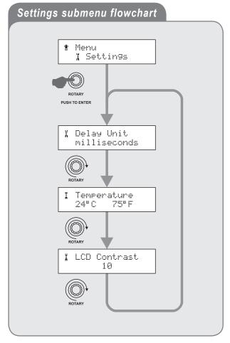
Once the first submenu item is displayed, the rotary encoder can be used to step through the others; to select an item, press Enter while it is displayed.
