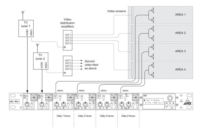
Audio to video synchronization error (also known as lip-sync error) can be a significant problem in audio-visual installations when digital displays or projectors are used.
